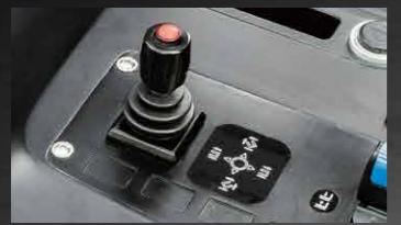
**The thumb switch and the cross handle make the operation light and comfortable.**
